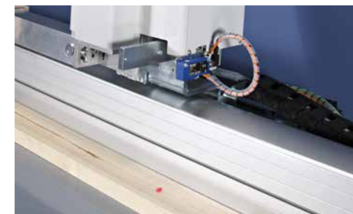
Close-up of pusher with workpiece measurement sensor
