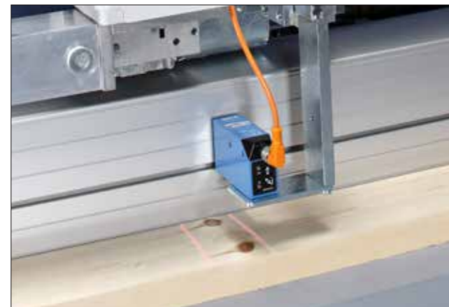
Video camera for identifying defects or knots, with reading of chalk marks.
