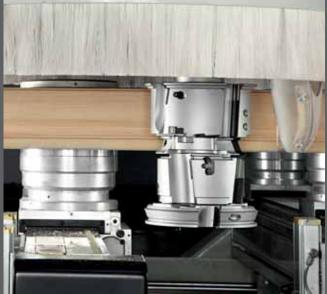
Prisma allows machining up to 10 degrees below the horizontal axis.
