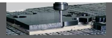
The directly machined worktable guarantees lasting absolute precision and perfect flatness thanks to its high level of rigidity. Also ideal for machining plastics, resins and light alloys.
