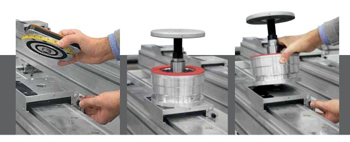
Switching from clamps to suction cups and vice versa is fast and practical. The quick coupling perfected by SCM allows operators to switch at the press of a button, without the need for external tools.
